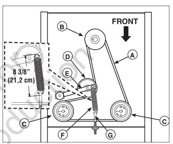
Figure 48. Hydraulic Pump Drive Belt Replacement A. Pump Drive Belt
